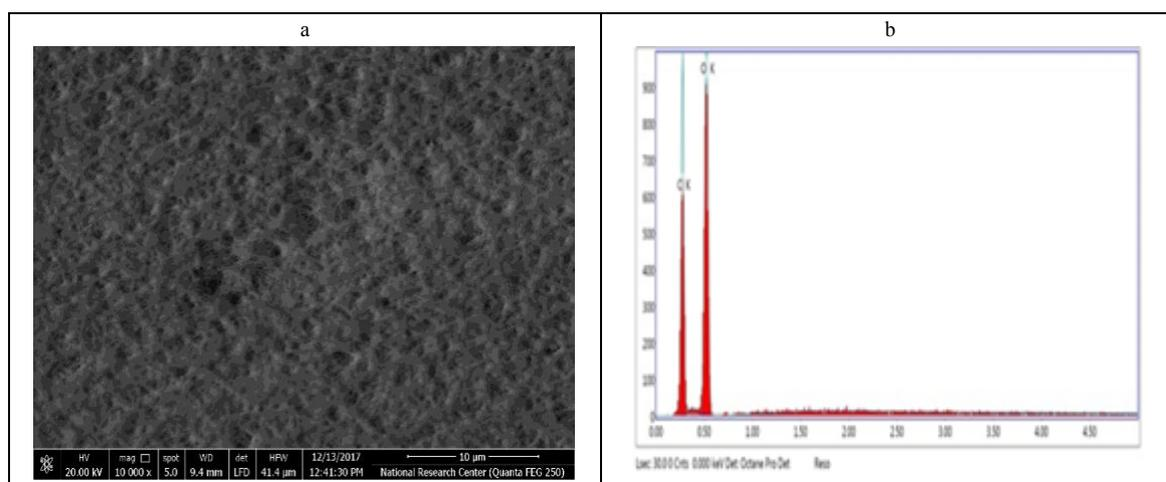
**Figure 1. SEM image (a), with EDS spectra (b) for the polycarbonate filter (blank) before sampling.**
