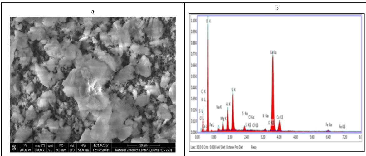
**Figure 5. SEM image of calcium rich particles (a) and EDS spectra (b) in TPM samples.**
