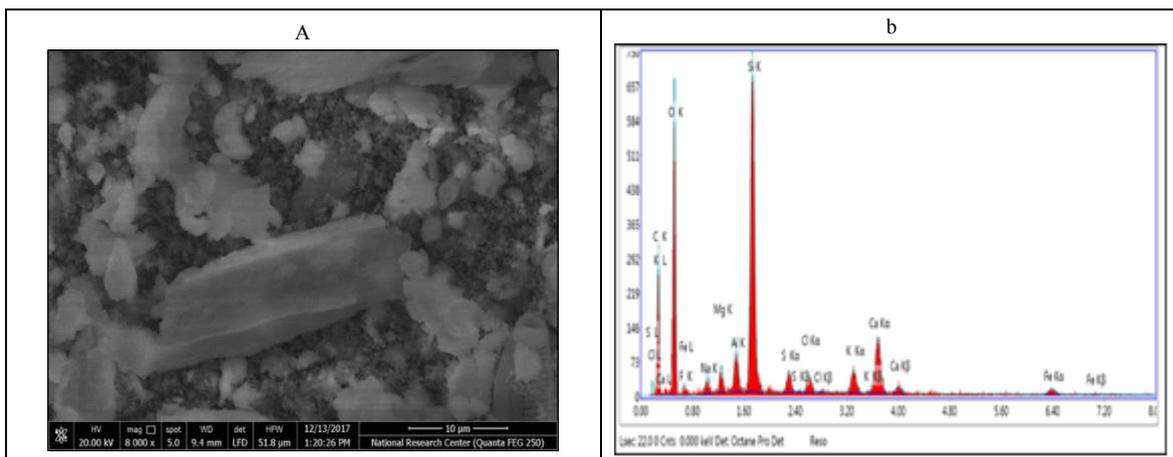
**Figure 4. SEM image of Aluminium silicate particles (a) and EDS spectra (b) in TPM samples.**
