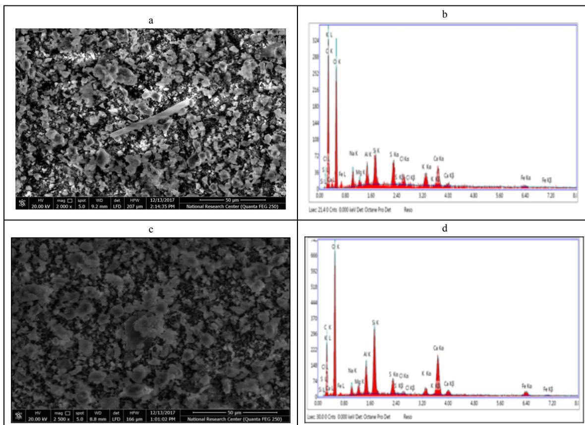
Figure 2. SEM image (a), with EDS spectra (b) of a loaded filter in winter season. Also, SEM image (c), with EDS spectra (d) of a loaded filter in summer.
